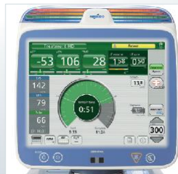
15 inch flat touch screen with wide viewing angle. 4 colored status display on top of the screen with 360° visibility.
